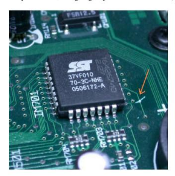
Step 3, Place the Socket/PROM assembly over your original PROM as illustrated below, it should fit nice and tight, should it fit loosely over the PROM it will not work and you will have to get a different socket assembly- some sockets will not fit tight using them backwards over the original prombe warned.
